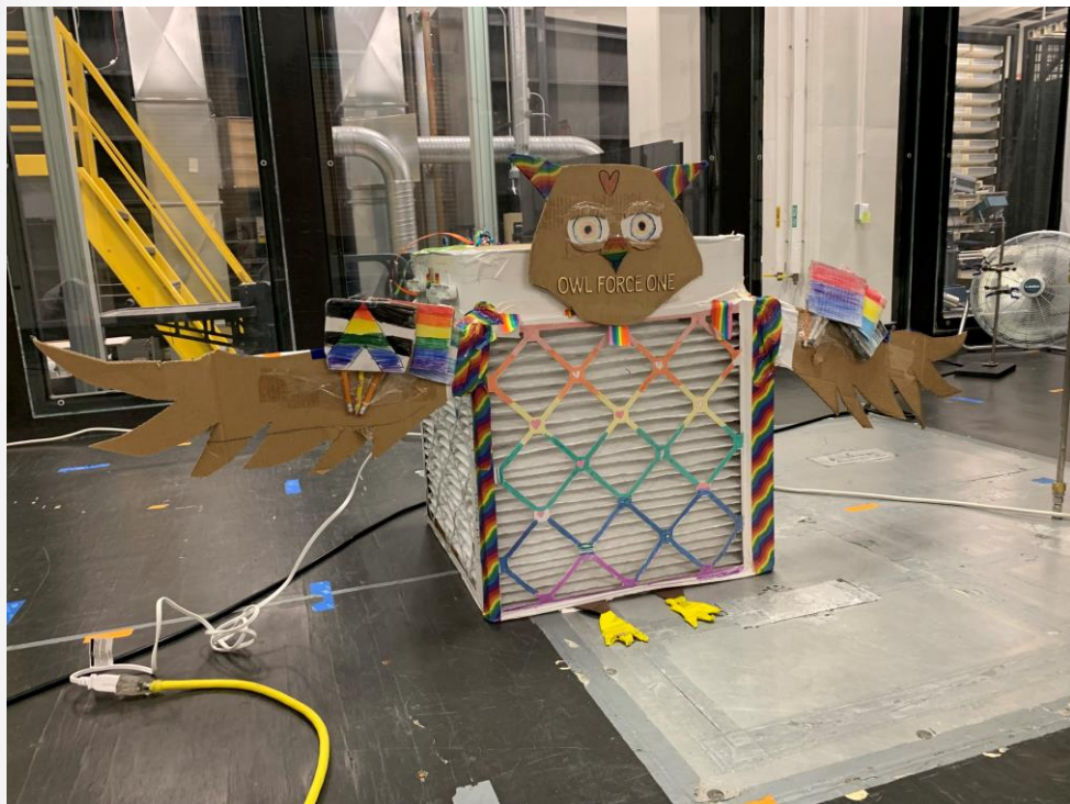
(Left) Owl Force One, built by 5 th grade class in Connecticut. (Right) EPA-assembled Corsi-Rosenthal (CR) Box, constructed from 20x20x2 inch MERV-13 filters. A new CR Box was used for each test.
